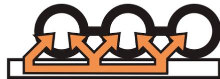
The 'heat trap' design enables stored energy to be radiated directly from the roof to the water channels.
